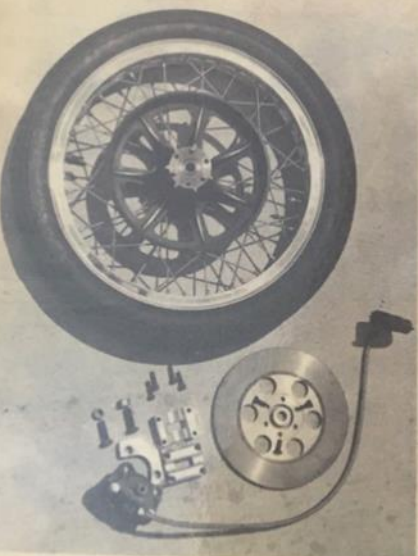
This complete wheel and brake assembly weighs only thirteen and a half pounds.
