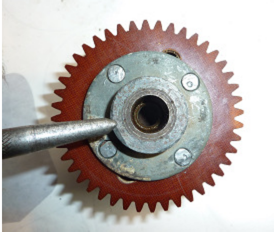
21. Make four punch marks at the join between the collar and sleeve for additional security.
