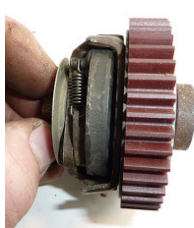
22. Final check. Soak in oil before fitting. This job usually takes me about two hours so you can easily come home from work, have your tea, fit the new gear and.....
